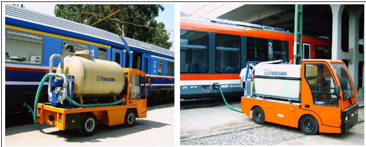
*Example of mobile carriages used for water tanking and sewage removal.*
