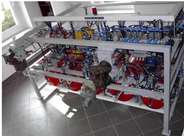
*Fig. 25. Exemplary brake valve test station.*
