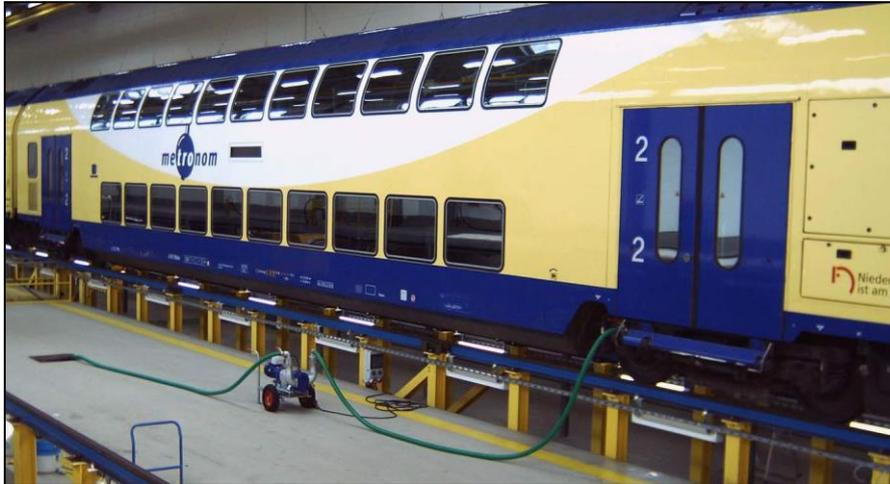
*Exemplary use of a mobile pump for faecal sewage removal from a car. In this case, it is necessary to provide a relatively close access to the sewage drain designed to take over faecal sewage.*
